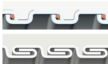
Square-Locked Design with integral bonding wire 3/8" - 1-1/4"
