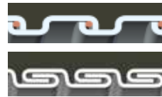
Square-Locked Design with integral bonding wire 3/8" - 1-1/4"
